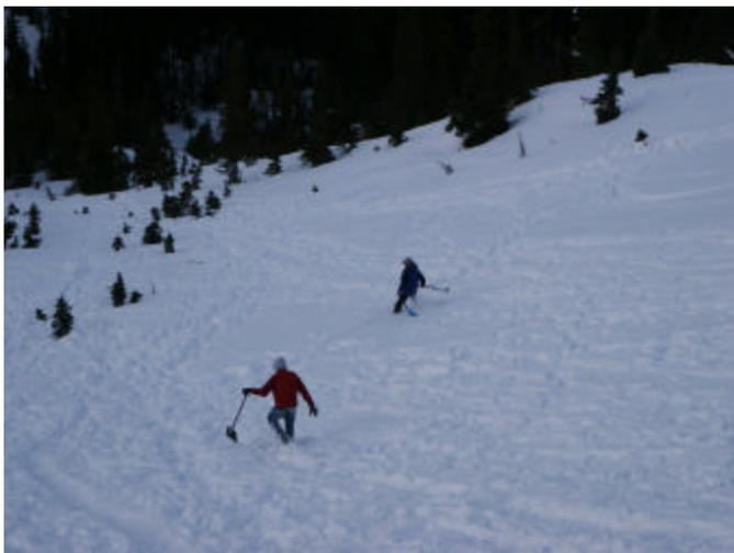
The improper way of testing the stability of the snow slope.
